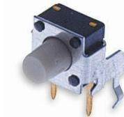
The pushbutton can only be inserted one way. The actuator (that you press) faces away from the PCB. It snaps into place and will stay put while you solder it. Make sure it is fully inserted and seated flush against the PCB.
