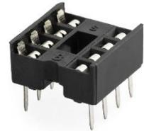
There is one 8-pin socket and three 14-pin sockets. Sockets are marked with a small notch that must line up with the outline on the PCB. Once the socket is soldered in place, the PCB outline will not be visible, so it is important that the sockets are oriented correctly in order to ensure that the chips are inserted into the sockets correctly.
