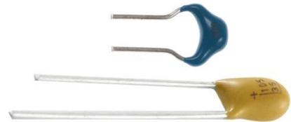
Ceramic capacitors are small tan or blue blobs. Their value is marked on them with a three-digit code. The marking is rather tiny, so you may have to use a magnifying glass to read them. It does not matter which lead goes in which PCB hole.
