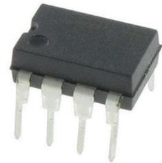
The pins of the chips come from the factory a little bit splayed out, not pointing straight down. You may need to bend them inward a little before you insert them. Hold the body of the chip and rest all of the pins on one side against the table top and gently press down just a little bit. Then do the other side. If the pins do not line up well with the socket, repeat the straightening procedure.
